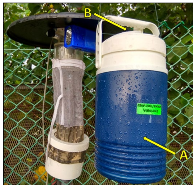
Figure 2. A CDC miniature light trap used in the study to trap field mosquitoes. The blue insulated container was filled with dry ice during the operation of the trap (arrow A), and small holes (arrow B) at the top allowed the released of CO 2 gas to be dispersed by the fan of the trap.
